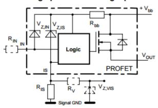
$R_{bb}$  = 120  $\Omega$  typ.,  $V_{Z,IN}$  =  $V_{Z,IS}$  = 74 V typ.,  $R_{IS}$  = 1k $\Omega$  nominal. Note that when over voltage exceeds 79 V typ. a voltage above 5V can occur between IS and GND, if  $R_V$ ,  $V_{Z,VIS}$  are not used.
