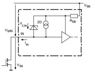
When the device is switched off (I<sub>IN</sub> = 0) the voltage between IN and GND reaches almost V<sub>bb</sub>. Use a bipolar or MOS transistor with appropriate breakdown voltage as driver.
