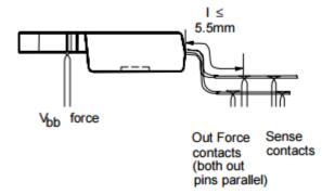
Typical RON for SMD version is about 0.2 m $\Omega$  less than straight leads due to I = 2 mm
