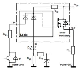
$R_V \ge 1 \text{ k}\Omega$ ,  $R_{\text{IS}} = 1 \text{ k}\Omega$  nominal. Add  $R_{\text{IN}}$  for reverse battery protection in applications with  $V_{bb}$  above  $16V^{18}$ :
