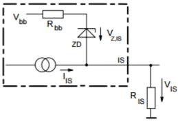
$V_{\rm Z,IS}$  = 74V (typ.),  $R_{\rm IS}$  = 1 k $\Omega$  nominal (or 1 k $\Omega$  /n, if n devices are connected in parallel).  $I_{\rm S}$  =  $I_{\rm L}/I_{\rm Hilis}$  can be driven only by the internal circuit as long as  $V_{\rm out}$  -  $V_{\rm IS}$  > 5 V. If you want measure load currents up to  $I_{\rm L(M)}$ ,  $R_{\rm IS}$
