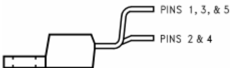
Figure 37. Bent, Staggered Leads 5-Lead TO-220 (T) Package LM2576T-XX Flow LB03 or LM2576HVT-XX Flow LB03 See Package Number NDH0005D
